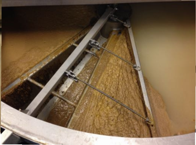
Ozonesystem and float material at Adoxpol system installed at Marine Harvest Fish feed Factory in Norway
